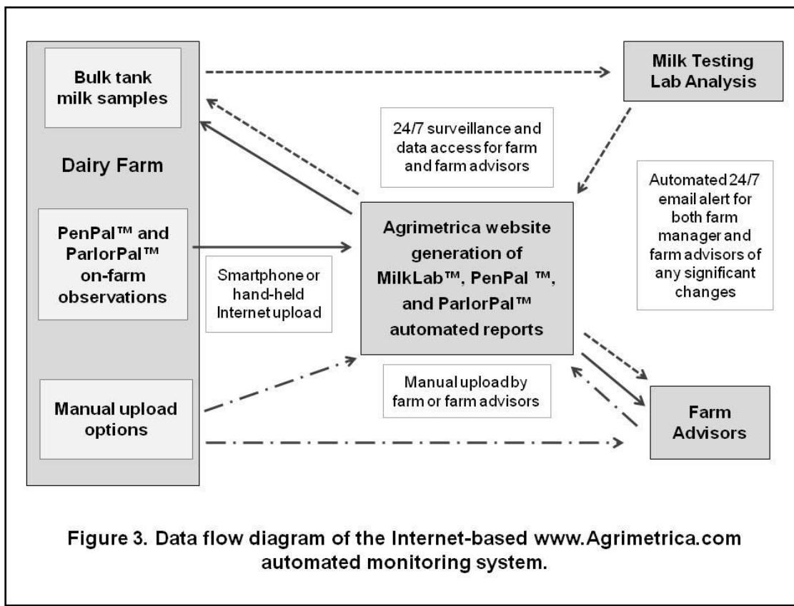
**Figure 3. Data flow diagram of the Internet-based [www.Agrimetrica.com](http://www.Agrimetrica.com) automated monitoring system.**
